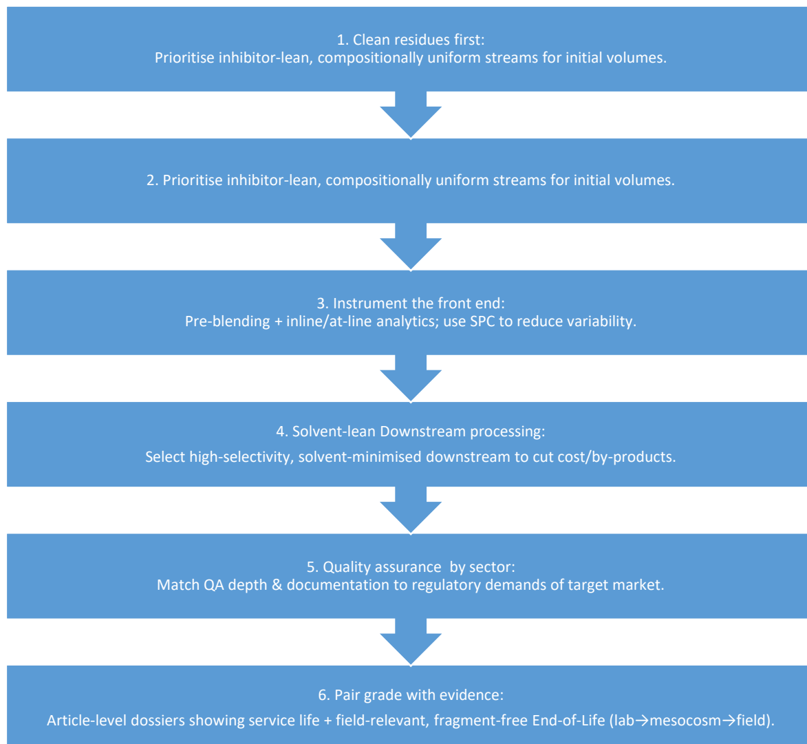
Figure 18: Framed process' market-entry workflow for residue-based PHAs (Own compilation by Ecozept).
