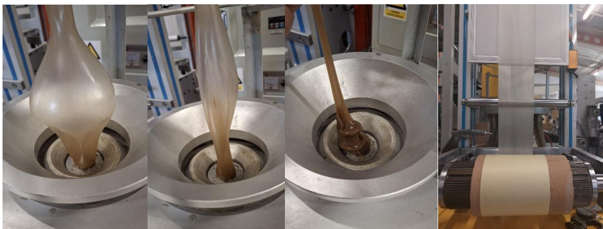
Figure 25. Film (blow) extrusion of PBSA/PHBV UNIVR material (top) and PBSA/PHBV PBM (bottom) – 8 th trial
