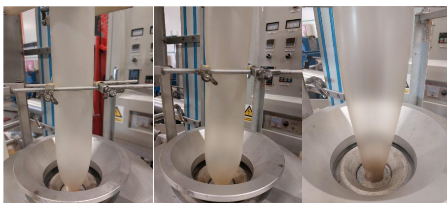
Figure 26. Blow extrusion of MI3/PHBV Tianan Enmat Y100P (left), MI3/PHBV PBM (middle), and MI3/PHBV UNIVR (right) – 8 th trial
