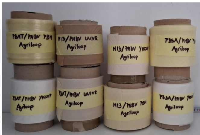
Figure 27. Film rolls of materials prodced within the 8 th trial
