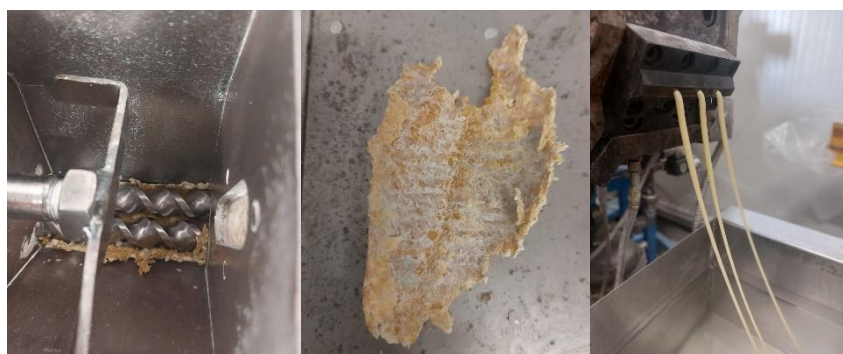
Figure 21. Compounding of PBAT/PHBV PBM – 8 th trial
