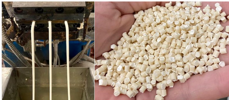
Figure 10. Compounding process of bio-based benchmark “MI3” – 3 rd trial
