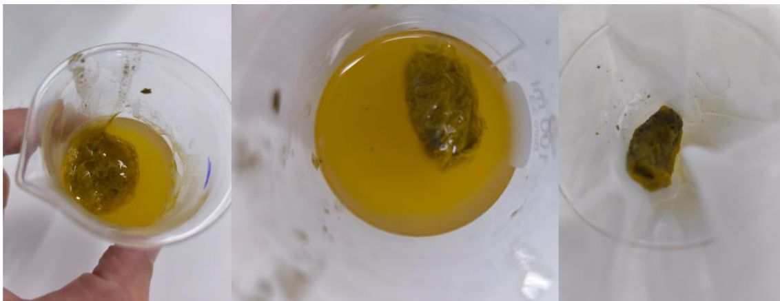
FIGURE 48 : PHA CONDENSATION. A) AND B) DEMI WATER IS ADDED WHILE AGITATED AND A GUMMY SOLID APPEAR; C) THE SOLID IS SEPARATED FROM THE LIQUID USING A NYLON MESH OF 75 MICRONS
