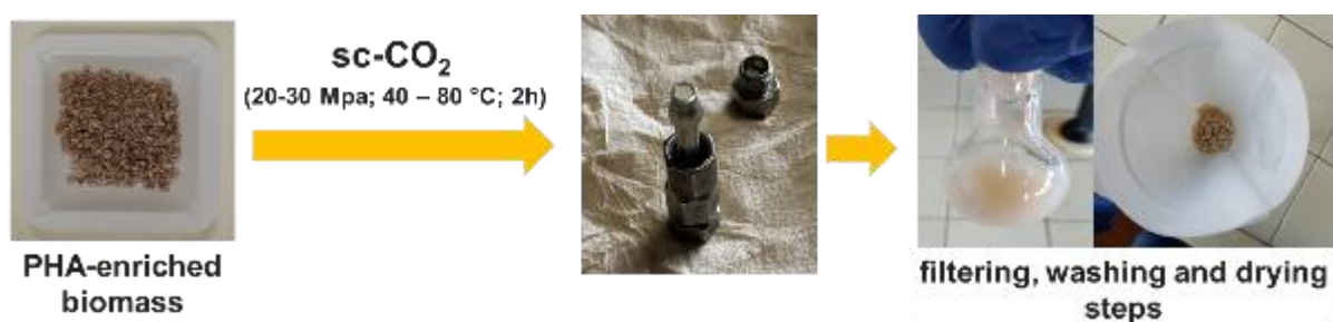
FIGURE 27: SFE SCHEMATIC PROCESS OF THE RAW BIOMASS ENRICHED INTO PHA
