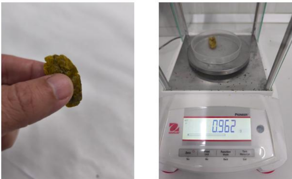
FIGURE 49 : FINAL PHA PELLET YELLOW PHA PELLET INDICATED CERTAIN IMPURITIES AND TST GAVE A TOTAL PURITY OF 95%.
