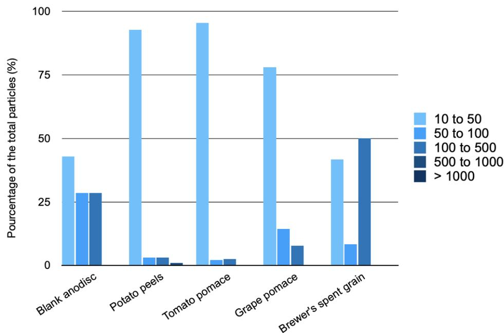
**Figure 11:** Size distribution of microplastics determined with ImageJ®
