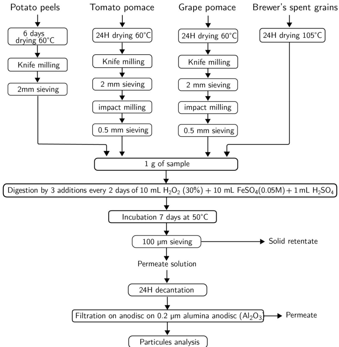
**Figure 1:** Experimental approach applied to the analysis of the contamination of agricultural residues by plastic particles
