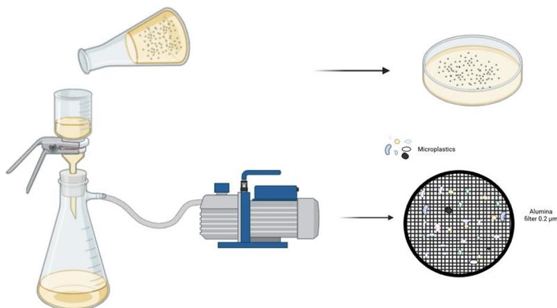
**Figure 9:** Second filtration and separation of digestate from sediments
