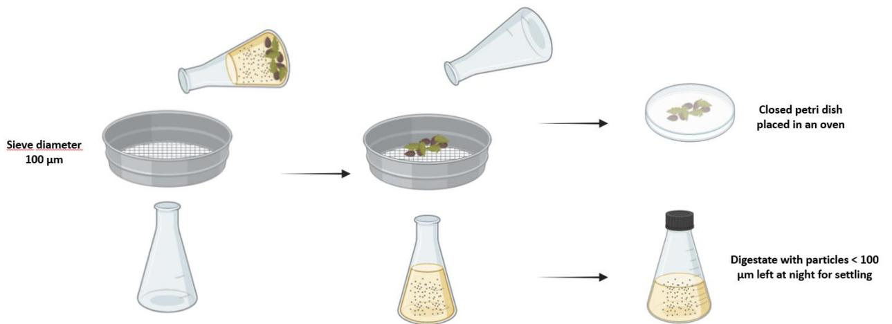
**Figure 5:** First filtration of the digestion solutions using a 100 µm sieve
