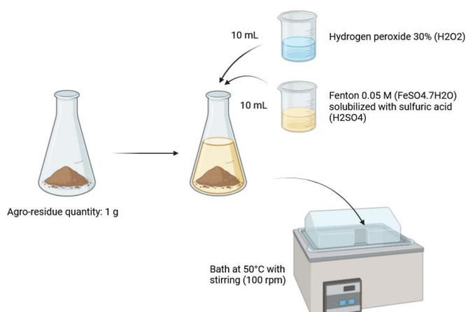
**Figure 4:** Digestion procedure applied to residue samples
