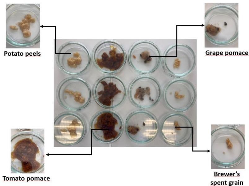
**Figure 6:** Non-digested part of the various agro-residues larger than 100 µm
